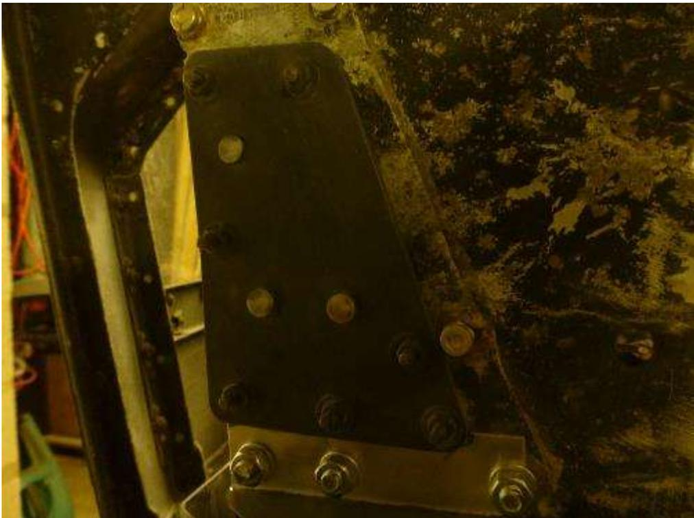
The space in front of the valve box already looks tight. However, there is still the shaft centre support (which also mounts the gun fire solenoids), another hydraulic feed line, the valve box links, the front part of each empty case chute and the armour to get into this area.
