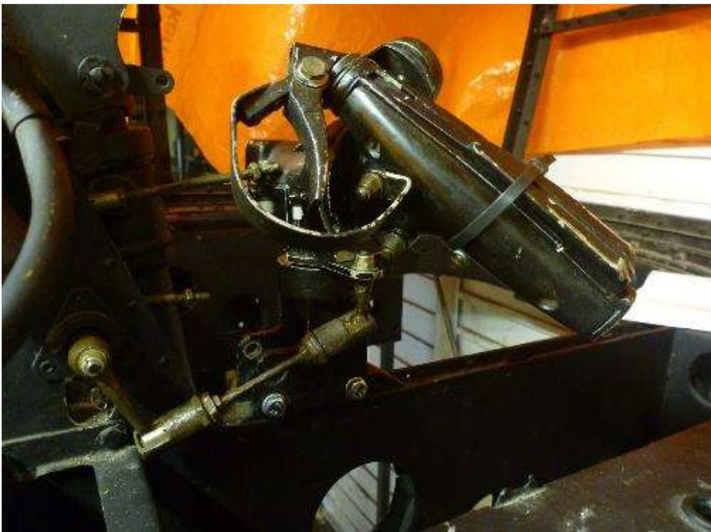
Next month. Sort out these rods that join the control handles to the control shafts and produce a new shaft centre support and solenoid mount. The centre support and solenoid mount is also missing but, luckily, I have the remains of one from the FN5 to copy.
