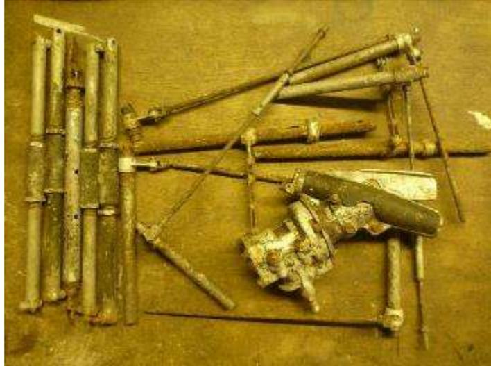
In short, the control system comprises of two control handles each of which can activate the hydraulics, rotate the turret, elevate the guns and fire the guns. All this is achieved with rods and levers in the wonderful, pre-electronic age!
