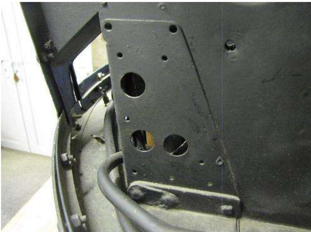
Whilst the left side support was present, the right side one was conspicuous by its absence. So, the first task was to make this assembly as it was needed to obtain the overall length of the control shafts.
