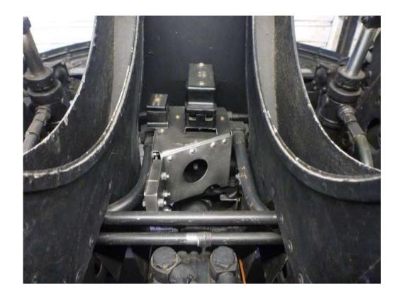
The right side control handle was finished off and then sprayed. In the FN-150 the guns were electrically fired and so both handles will need to have a firing micro switch fitted – I will need to try to find a pair of these and then produce their mounting brackets.
