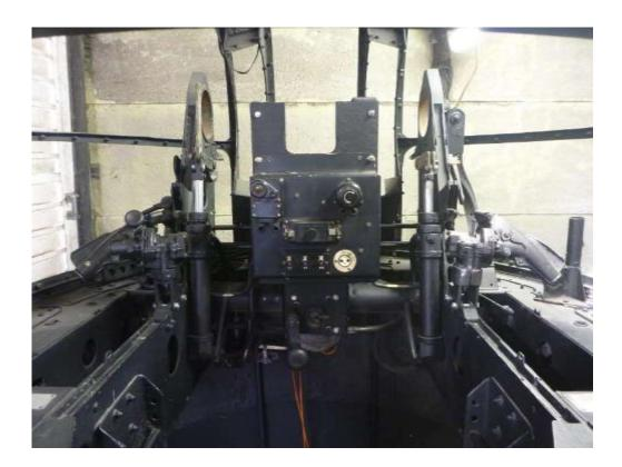
The Above Turret Ring Armour Plate was the next assembly to go into this, already overcrowded, area. Unfortunately, the two largest panels of this assembly are missing (see below) and if these cannot be found then they can be replicated.
