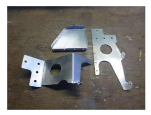
The bracket was then assembled, fitted, removed, tweaked about and then finally fitted onto the Valve Box. This took quite a while as I was keen to make this fit the final one. Once the bracket was in the Firing Relay could be fitted alongside its junction box, both of which have their own brackets. When the triggers are pulled, this relay closes and activates the two firing solenoids, the firing solenoids withdraw, pulling a Bowden cable which in turn fires the guns.
