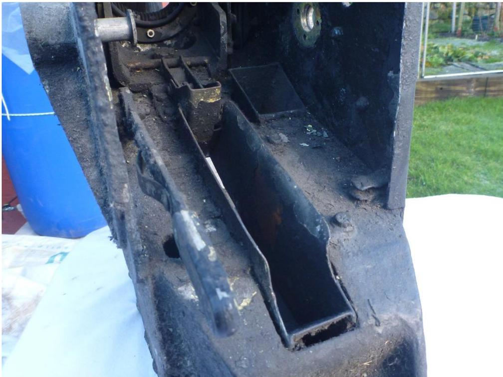
Once dismantled, the parts could be cleaned, inspected and then sprayed in preparation for re-assembly. Again, these will be dusted over in black before re-assembly and then finally sprayed again in their assembled state.
