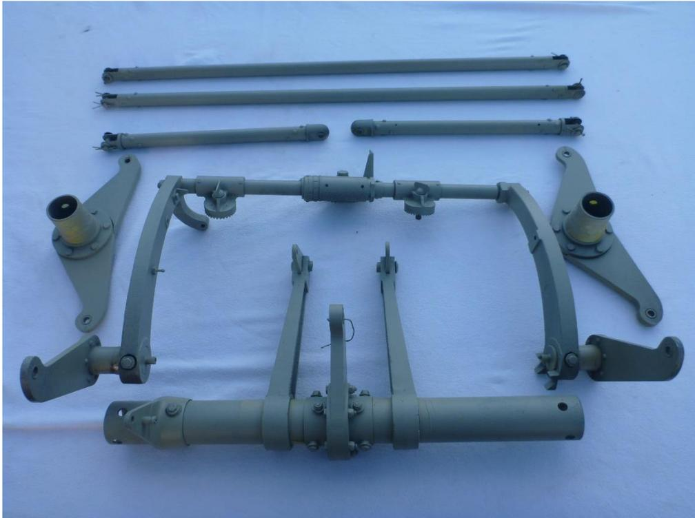
With the controls set to one side for the time being, attention turned to the gun cradles. These are complex assemblies and almost a project in their own right. Each has been subject to many previous layers of paint and, without exaggerating, in some areas the paint was up to  $\frac{1}{4}$  inch thick. It was decided to do these one at a time as, despite having the relevant Air Publications, it is always easier to have a complete example to copy.
