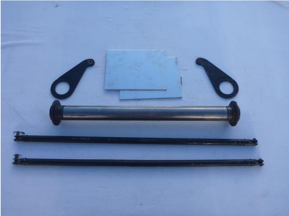
Seen above are some of the components of the display turret control system. The torque tube needs to be bolted onto the bearing ends and then the control levers fitted. The two alloy blanks are for the re-manufacture of the two missing control levers.
