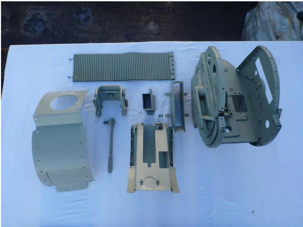
By this point, there are many assemblies awaiting spraying in black, however, the black paint has yet to arrive. Therefore, there was a useful period during which some time could be spent on the display FN82 Series 2 turret. The servo ammunition feed unit was completed and is now ready for painting. On the Series 2 turret the servo feed is an electrically driven unit as opposed to the hydraulic one on the Series 1.
