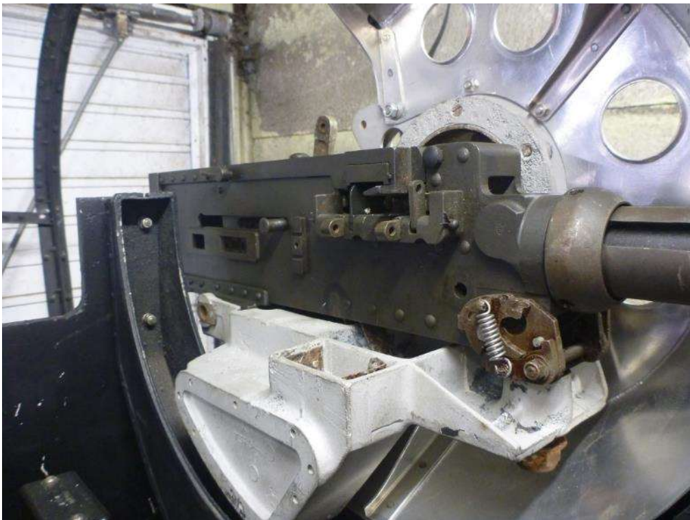
Visible here is the front Gun Mount with new springs.
