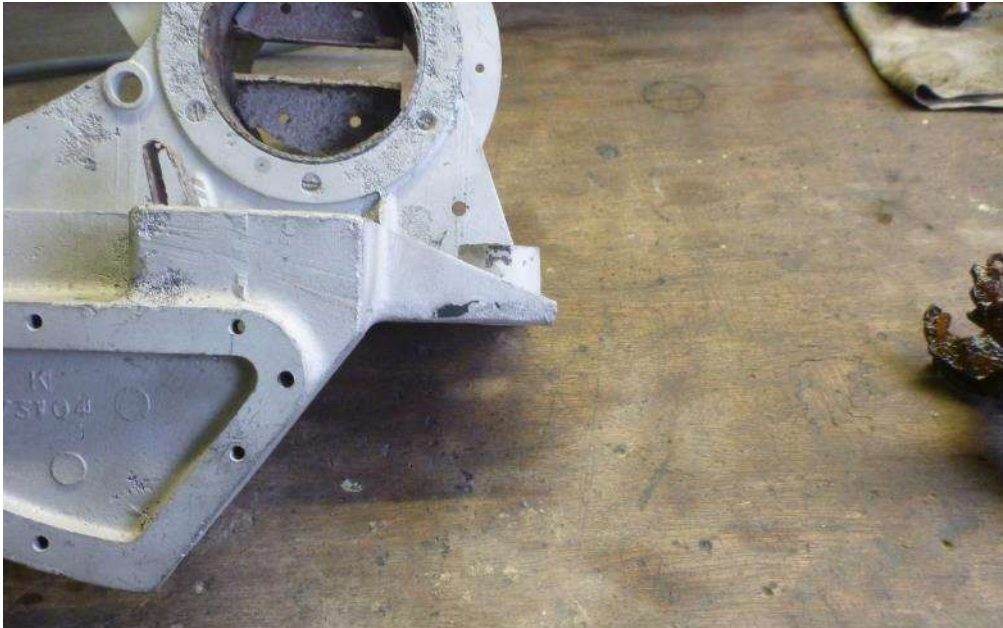
A view of the left side Gun Cradle showing the lack of Interrupter bracket
