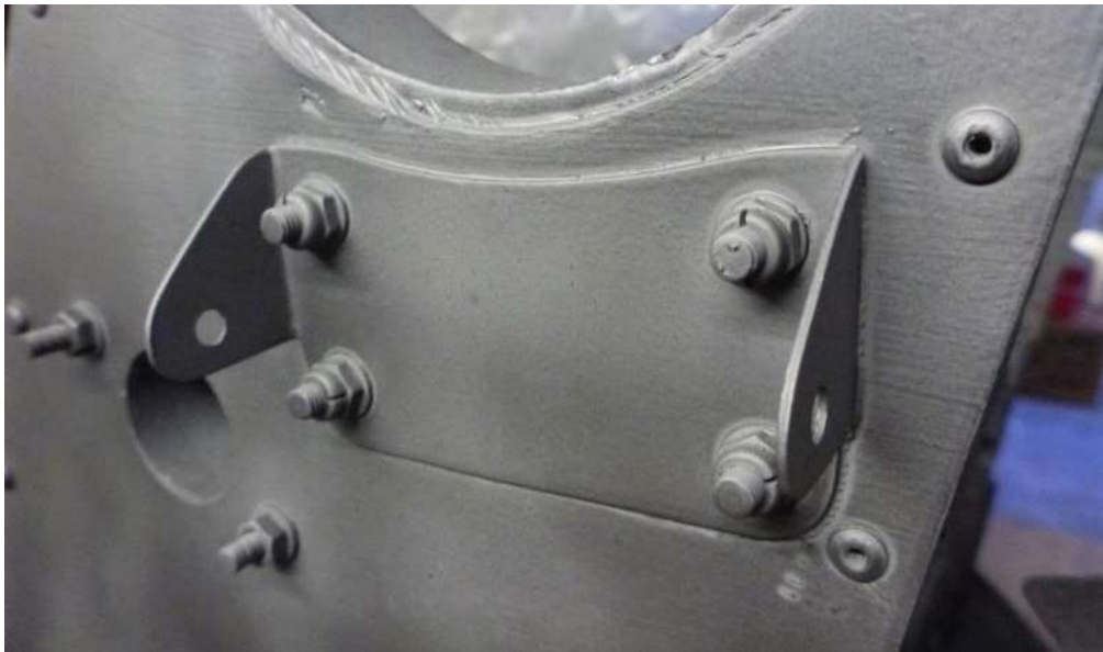
Ammunition rail top bracket – Again on the FN-5 for ease of photography
