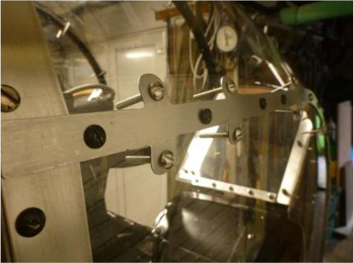
Several days work resulted in a complete turret cupola front half that just needs the cross frames fitting and their capping strips fitting at some point.
