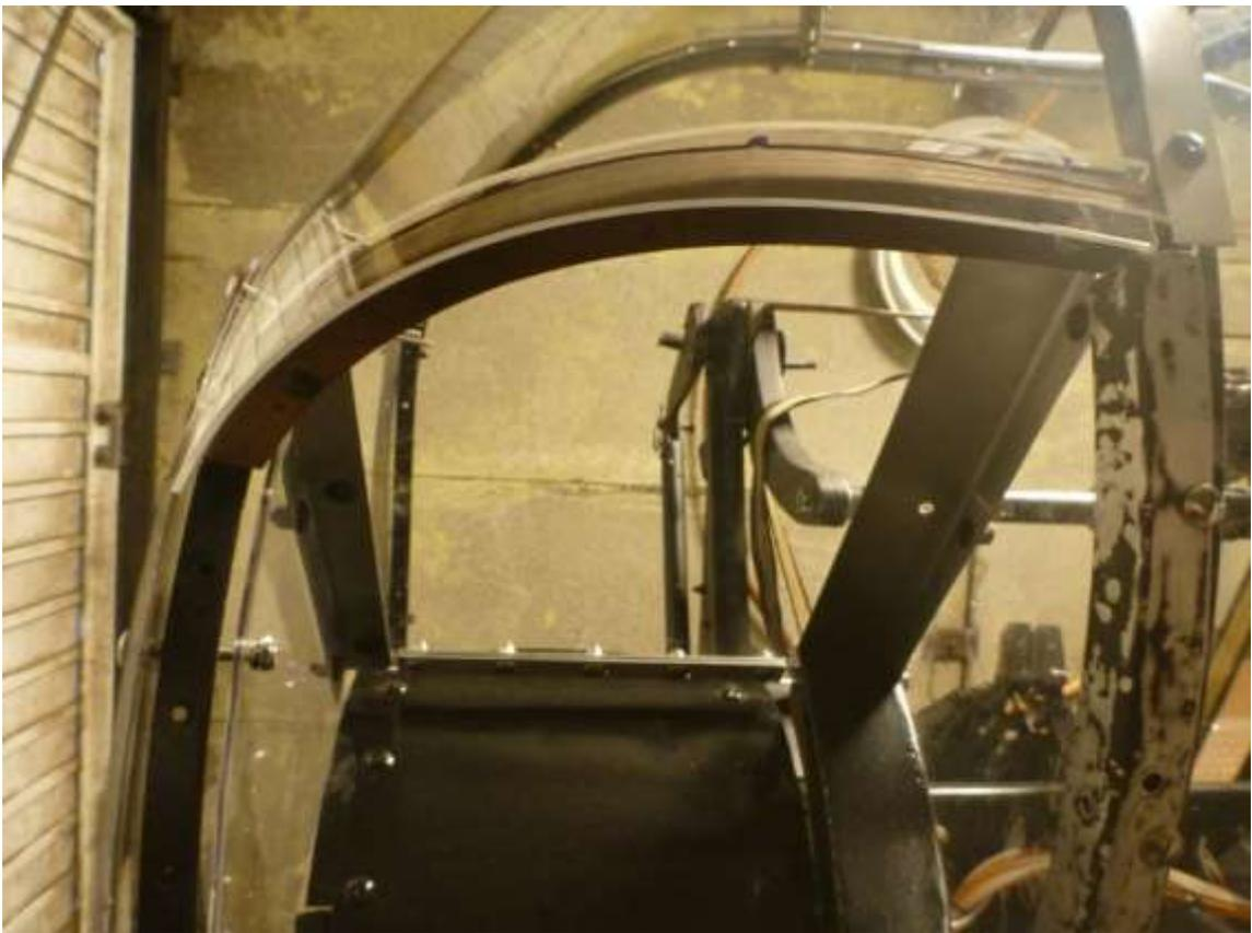
With the panels all made and positioned, the next task was the capping strips. No original capping strips were left on Just Jane's turret as the result of various restorations over the years. However, most of the bolt holes could be accurately worked out either from the pen markings on the curved panels or from original holes in the frames.
