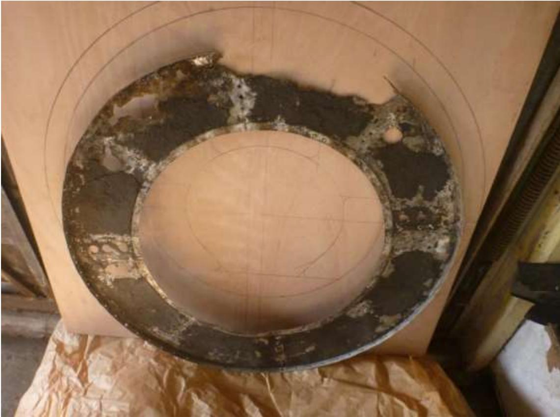
With the original drum sides fitted within a new build floor it was easy enough to mark the rivet holes and drill them. This was done with both new floor panels. The drum sides could then be grippered and then riveted to the floor.
